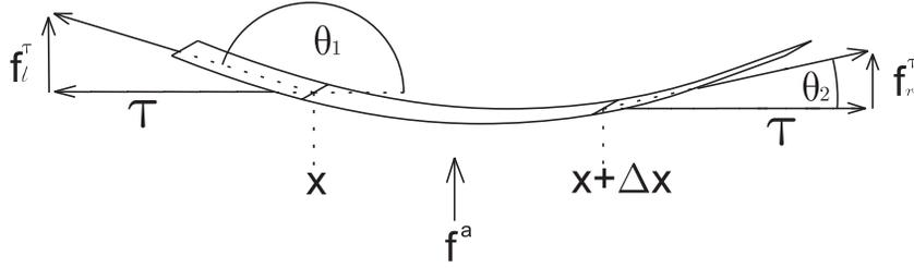
Figure 3: Forces acting on a small section of the membrane
